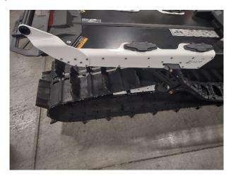
\*\* Note: Longer rivets are to be used when going through both the side panel and the Grab Bar side plate \*\*
