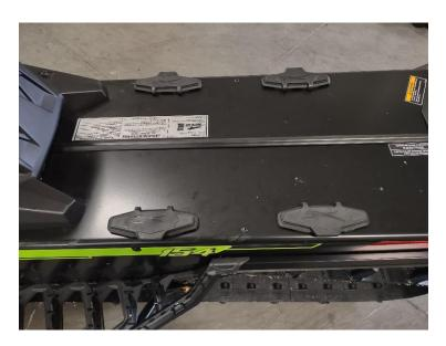
4. With the stock bumper removed, cut the plastic flap mount on the lines shown in blue. As straight as possible, so that no plastic extends past the side of the tunnel. There will be a triangle pointing up when complete.
