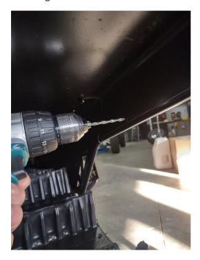
2. Remove the #20 Torx screws on the outside of the tunnel.
