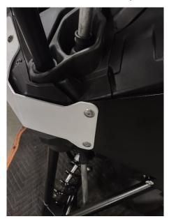
11. Drill 4 remianing holes in skid plate back near track. Rivet into place. 4 small head rivets.
