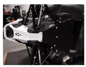
10. The two longest rivets join the Front Bumper "Bash plate" & the "Plastic Skid Plate" to the sled. These 2 rivets replace the Torx screws removed earlier on step 6.
