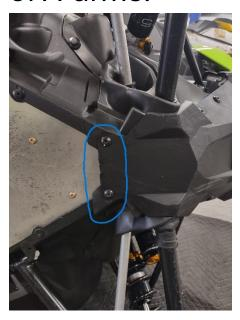
7. Rivet Grab Bar to Bash Plate, 4 small head rivets, 2 on each side.
