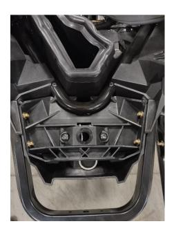
Remove Slip nuts from stock front bumper, Install slip nuts on Zbroz Front Bumper Grab Bar.
