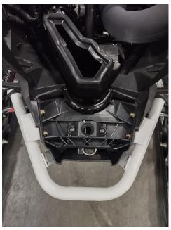
9. With Sled on one side, Place Plastic Skid Plate in position with some rivets to hold in place.
