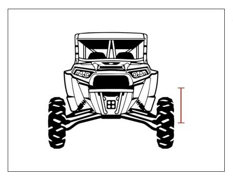
Due to payload options and initial ride height variances, the amount of preload is a base figure. Final ride height dimensions may vary in accordance to original vehicle ride height. Always measure the vehicle ride height prior to beginning installation.
