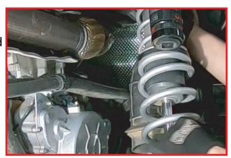
Disconnect lower shock bolt from trailing arm. Swing lower shock rearward and out.
