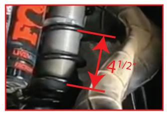
Align or clock lower coil end of new tender spring to upper coil end of new main spring. This reduces spring deflection.
