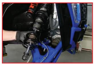
Install lower OEM spring retainer by reconnecting lower shock bolt to a-arm. Push down and hold a-arm to fully extend internal bump stop spring.
