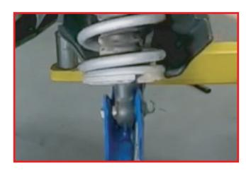
Push up on spring stack to remove OEM lower spring retainer.
