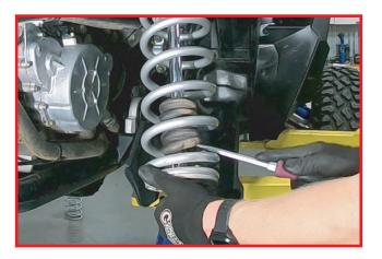
Rotate OEM spring stack and preload ring counter clockwise to the top of the threaded shock body.
