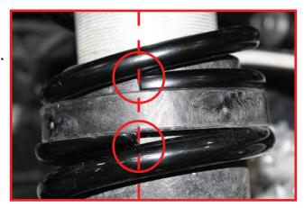
Positon cross over ring so that there is a 3/4" to 1" gap between bottom edge of cross over ring and top edge of spring divider. Tighten allen screws.
