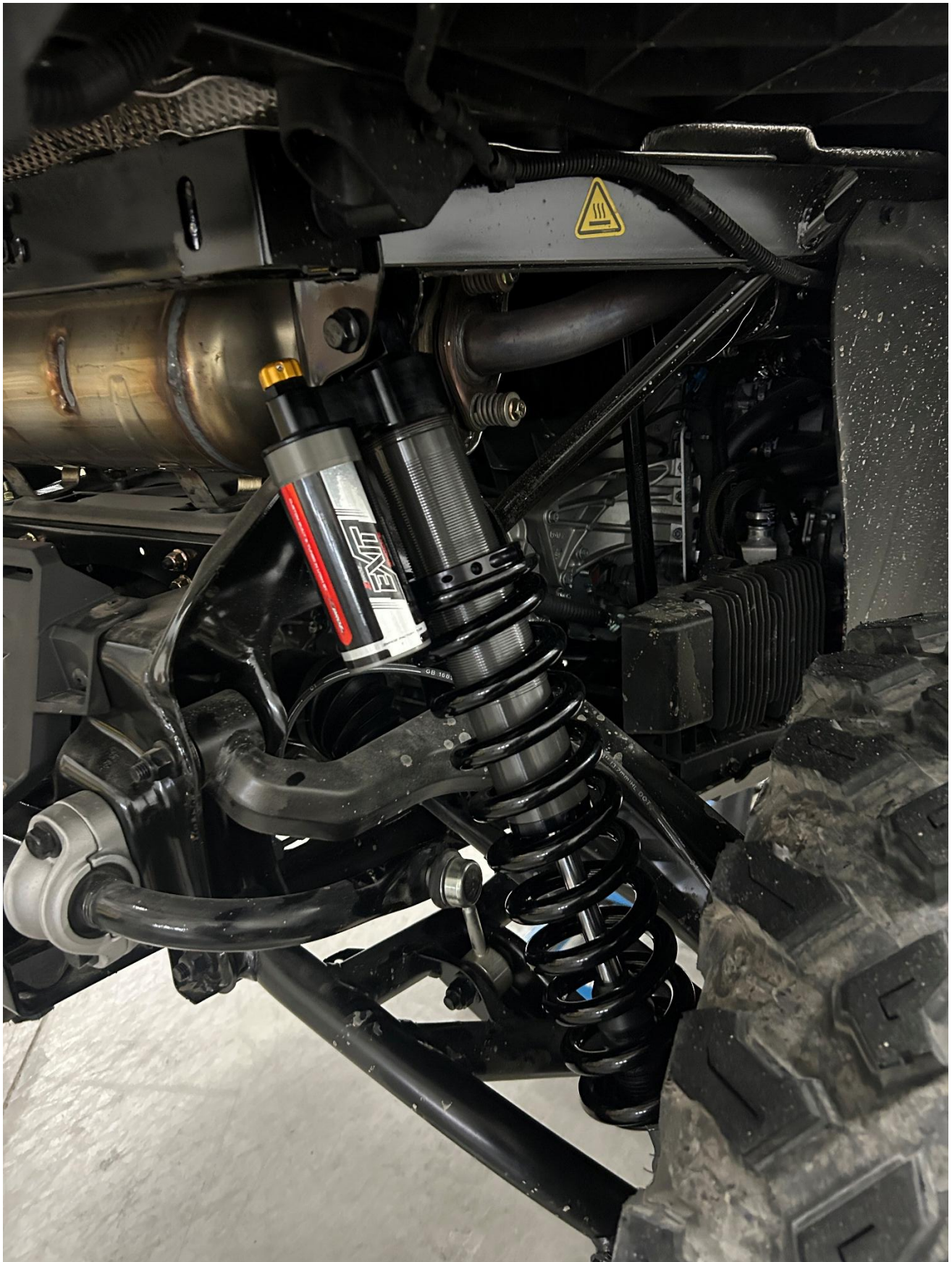
Passenger side rear shock installed
